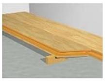
4. Place the floorboard at an angle against the first floorboard in the previous row, push forwards and press down at the same time, place a wedge under the board.
