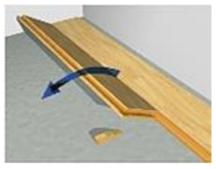
3. Start the next row with the piece left over from the previous row. It must be at least 50cm long, if the piece is too short start with a new board cut in half. Always ensure the end joints are staggered at least 50cm.
